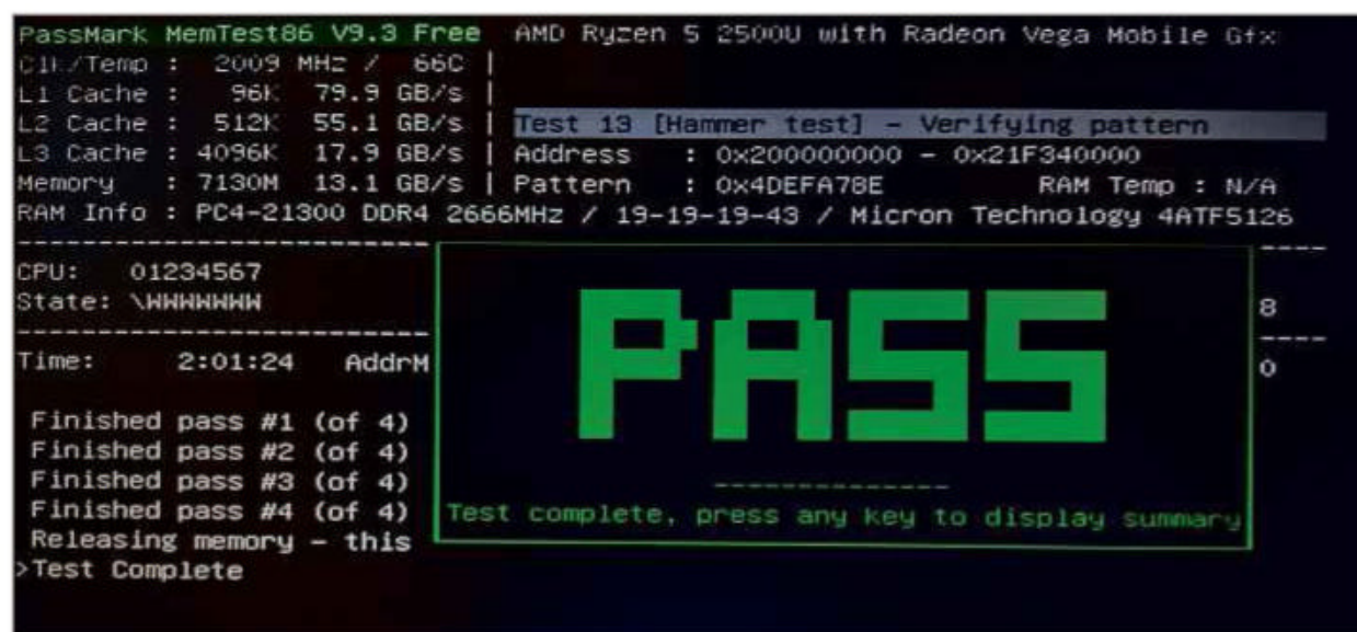
MemTest86 tests your PC thoroughly for bad memory but takes a long time to run
